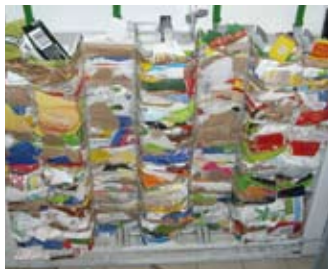
Volume reduction of packaging material by up to 95%
