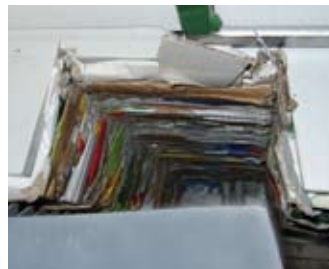
Special profiles form a recess in the bales
