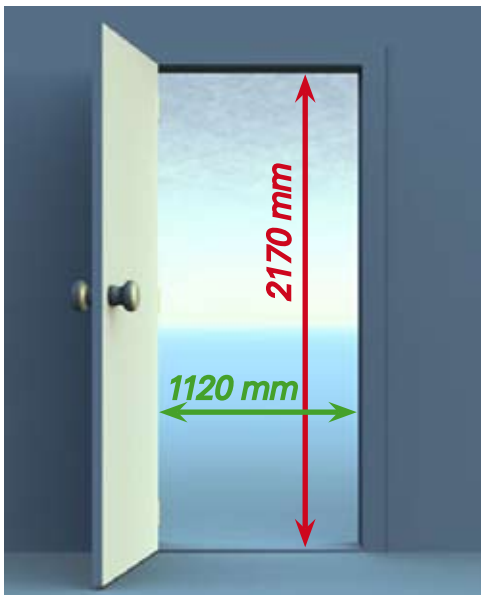
minimum sizes of the doors / passages
